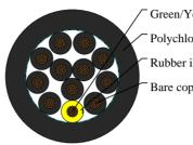
Green/Yellow wire Polychloroprene rubber outer jacket Rubber insulation Bare copper conductor
